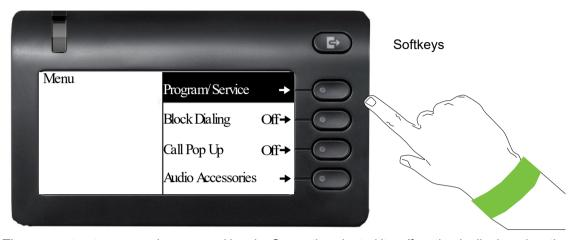
The menu structure comprises several levels. Currently selected item/function is displayed on the left side of the screen while options for this are listed as menu items on the right side of the screen. An arrow next to an entry indicates additional options for this entry.
