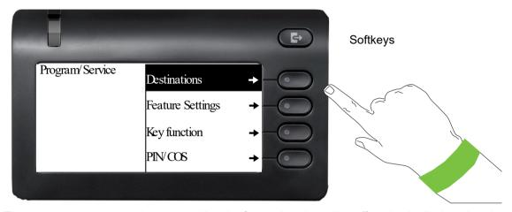
The menu structure comprises several levels. Currently selected item/function is displayed on the left side of the screen while options for this are listed as menu items on the right side of the screen. An arrow next to an entry indicates additional options for this entry.
