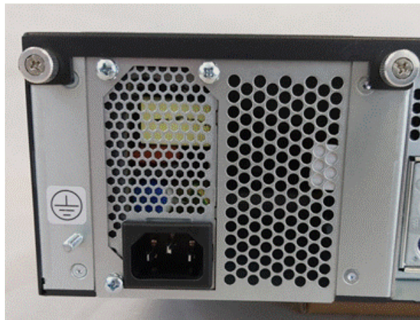
Figure 8: OSB 550- PSU 250W AC with single AC input power socket
