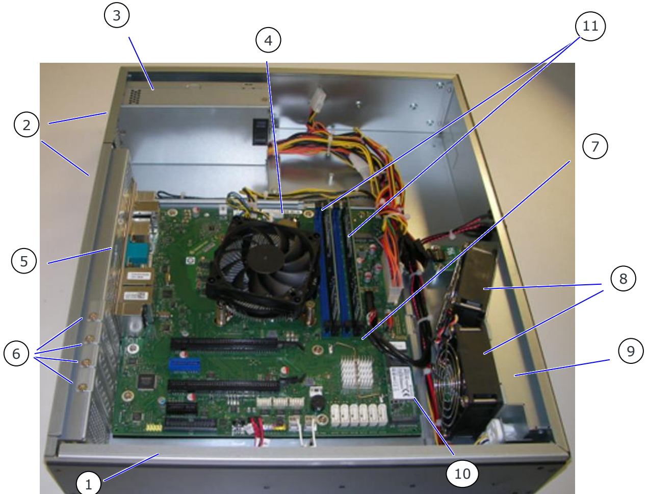
Figure 10: Configuration with micro-ATX mainboard and low profile expansion cards
