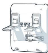
4. If your LAN does not have PoE (Power over Ethernet; ask your administrator), then you need to use a power supply connected to the power jack ③.
