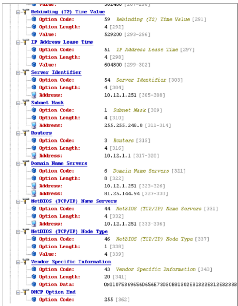
Figure 13: Example of a DHCP Acknowledge (Omnipeek Trace)
