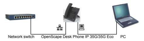
Using this connection option saves one network port for each switch used and requires fewer or shorter network cables when arranged correctly.
