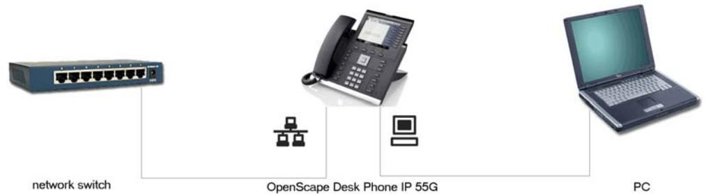
This type of connection allows you to save one network connection per switch, with the advantage of less network cables and shorter connection distances.
