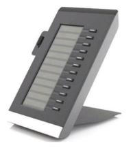
The diagram shows an OpenScape Key Module 55 for OpenScape Desk Phone IP 55G.
