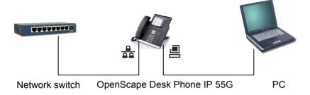
Using this connection option saves one network port for each switch used and requires fewer or shorter network cables when arranged correctly.
