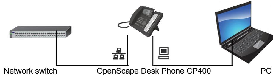
Using this connection option saves one network port for each switch used and requires shorter network cables.
