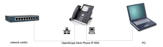
This type of connection allows you to save one network connection per switch, with the advantage of less network cables and shorter connection distances.
