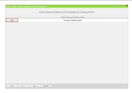
6. Enter the lowest DDI number in the range provided by BT into the **Internet telephony station** box. This number should be entered in canonical format for BT WSIPT as shown in the screenshot (e.g. +442380170422).
