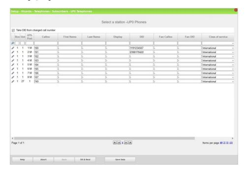
Click on the **Save Data** button after assigning all the required BT DDI numbers. Either click on the **OK & Next** button to continue with the wizard or close the window.
