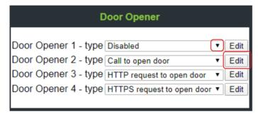
The configuration of the door openers depends on the selected control method. Fill in the required data and then click on Submit button.
