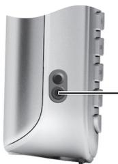
Once the plastic cover has been removed, you can connect a headset to the left side of the handset using a 2.5 mm jack.
