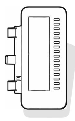
The KM410 is an optional key module attached and connected to the right side of the phone that provides an additional 16 illuminated and programmable function keys (see "Programmable function keys"  $\rightarrow$  page 62).
