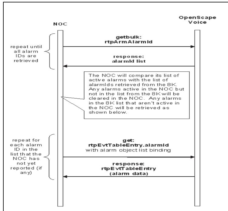
Figure 2 NOC Periodic Alarm Audit and Resynchronization
