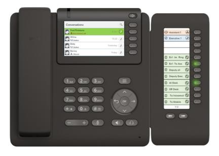
The leds at "Ex1: To Ass" and "At Desk" are highlighted.
