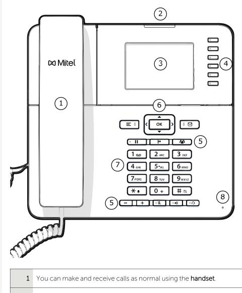
2 The **status LED** displays the phone connection status. Incoming calls and new voice mails are visually signalled via the notification LED.
