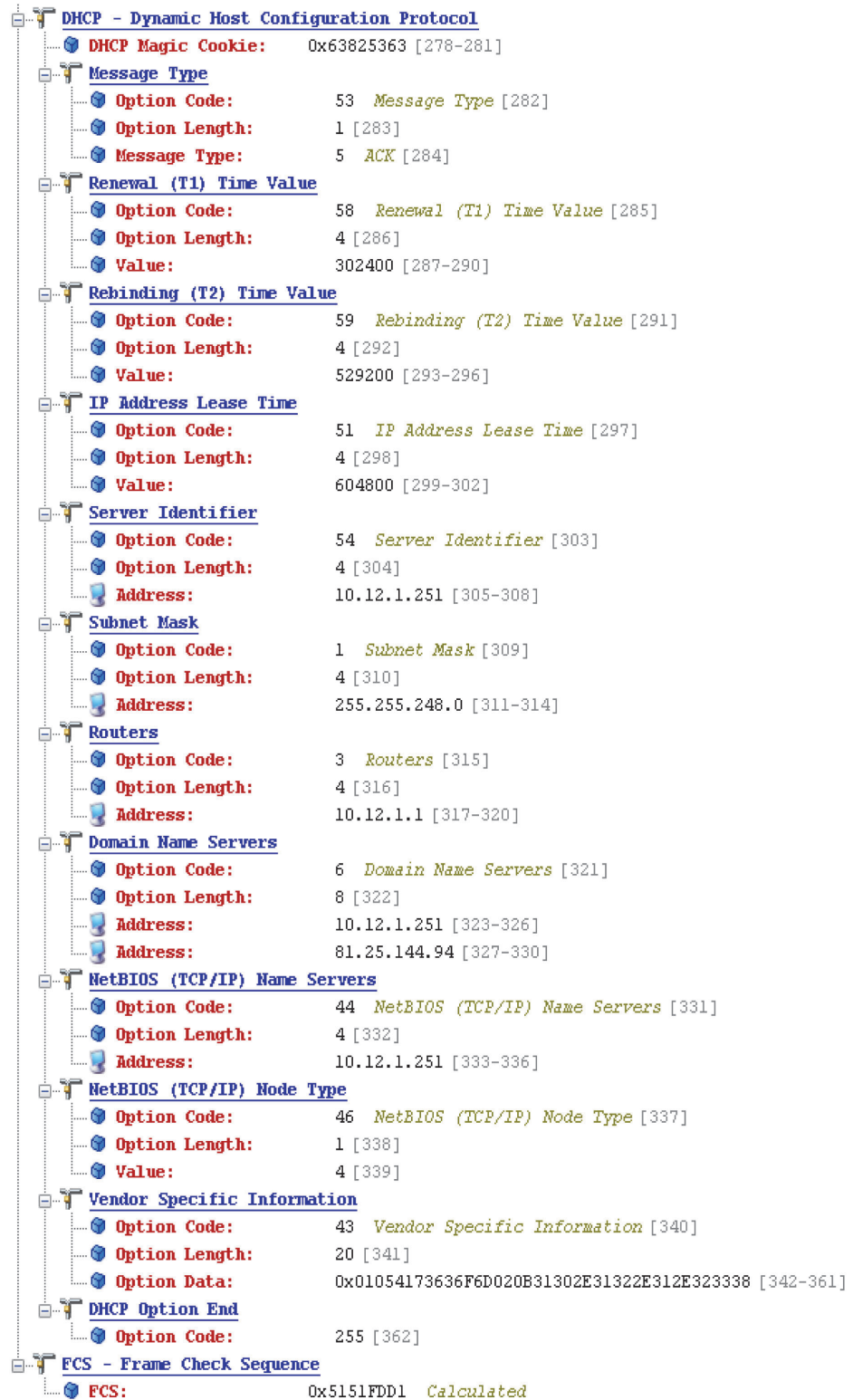
Figure 3 Example of a DHCP Acknowledge (Omnipeek trace).
