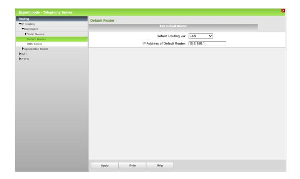
Traffic to the Orange SBCs e.g. 10.25.200.73 (nominal), 10.25.200.83 (backup) needs to be routed via the Network Access device.
