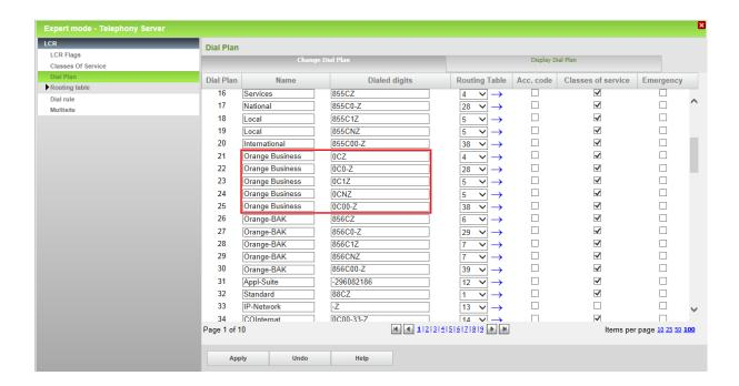
Open each routing table (e.g. 4,5,28 and 38) of the primary SIP trunk (i.e. Orange Business Services SIP trunking) and configure the backup trunk as the second entry with the same dialing rules (i.e. Orange-BAK).
