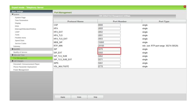
The internal SIP port should be set to a different port (e.g. 5070). Having internal and external port with the same value is possible but may lead to significant security risks.
