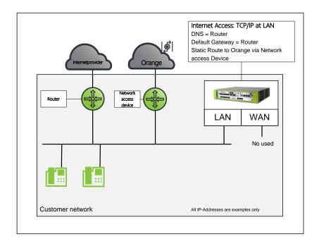
The OSBiz is connected via the LAN, to a Network Access device delivered to the customer as standard by Orange Business Services. This device will be added in the same subnet as the OSBiz subnet. The IP address of the device can be adapted by Orange, so that the Network Access device can be added in an existing voice VLAN of the OSBiz.
