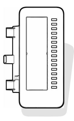
The KM410 is an optional key module attached and connected to the right side of the phone that provides an additional 16 illuminated and programmable function keys (see "Programmable function keys"  $\rightarrow$  page 65).
