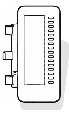
The KM410 is an optional key module attached and connected to the right side of the phone that provides an additional 16 illuminated and programmable function keys (see "Programmable function keys" > page 62).
