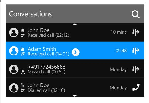
The conversations list is displayed on the screen. If the contact you want is not visible, select with the navigation keys or search by entering the phone number or contact name.
