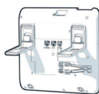
4. If your LAN does not have PoE (Power over Ethernet; ask your administrator), then you need to use a power supply connected to the power jack A ②.
