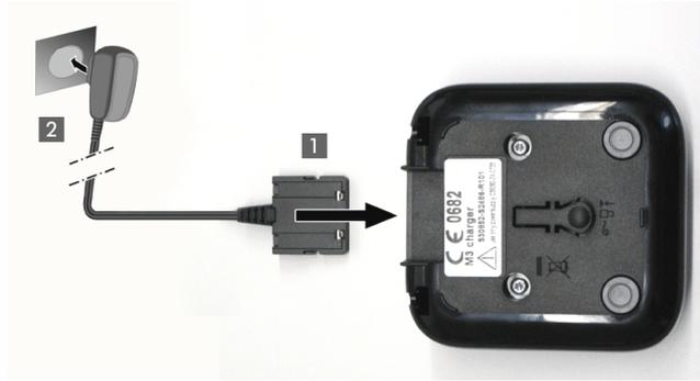
To disconnect the flat plug from the charger, press the release button and disconnect the flat plug.
