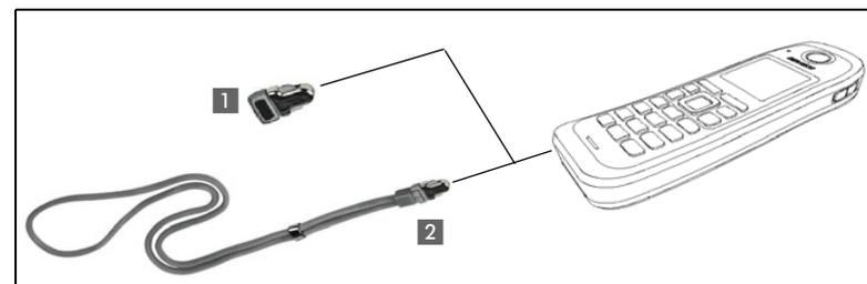
If you do not require the man down alarm function on the OpenStage M3 Plus or OpenStage M3 Ex Plus you can also use the connector without a cord as a dummy connector.
